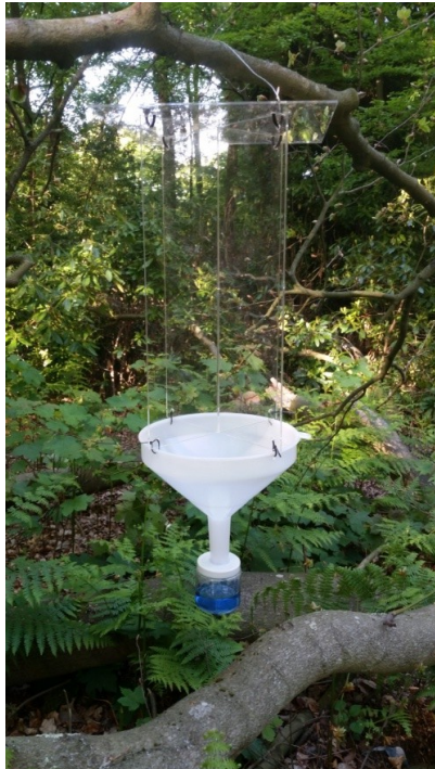
Fig. 1 Vane trap design used in this study.
